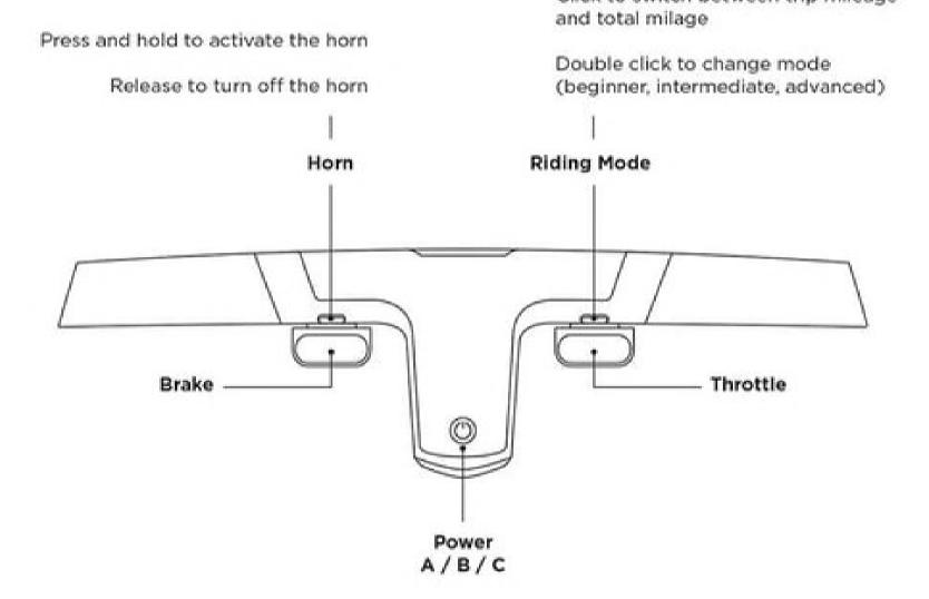
A Power (On/Off): Press and hold for 3 seconds. Motor will automatically turn off after 3 minutes if not in use.
