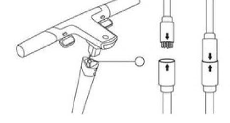
1. Press the hinge button down and fold the stem up.
